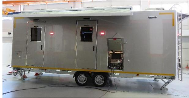
Engineering and lighting in whichever studio it is connected to. Recording and playback is done remotely on the Avid Airspeed in the Coronation Street studios’ CAR. All the studio wallbox signals are fed via fibre systems from the mobile gallery.
