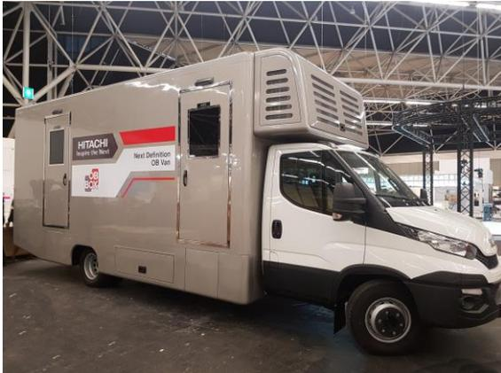
The OB-BOX™ comes in three different configurations which support four, eight and 12 production cameras. The option of a booth side extension adds further flexibility to unit sizing. In addition, an ability to connect two OB-BOX units in a cascade configuration adds more versatility and facilitates many different sizes of OB unit up to 20 camera mobile facilities.
